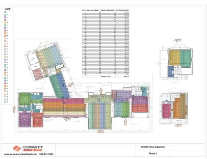
RadiantBoard EPS projects shall be provided detailed CAD drawings and schedules upon acceptance. System shall be installed as described in the current edition of the Ecowarm RadiantBoard Installation Manual.
