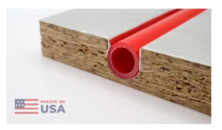
Ecowarm Radiantboard OSB is constructed using premium OSB substrate from the makers of \*AdvanTech® with a laminated aluminum surface. Panels are designed for application over subfloor or concrete. Our patented U-shaped groove locks PEX tubing into place without the need for screws or staples. The channel creates the pathway into which 1/2" PEX tubing is placed. Our system can be used under almost any finished floor covering.
