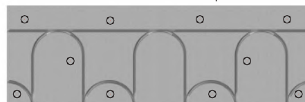
Top: Straight panel screw location. Below: Combo board screw pattern.
