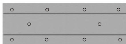
Top: Straight panel screw location. Below: Combo board screw pattern.
